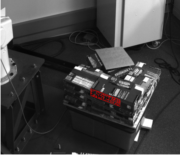
Figure 14. Rough Estimation of the Location of the Gap
