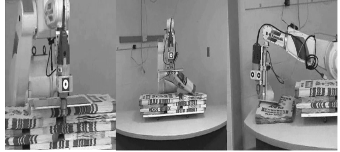
Figure 16. The Robot Inserted the Tool Into the Gap and Pick Up the Bags
