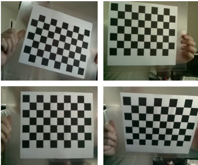
Figure 6. Camera Calibration Process
