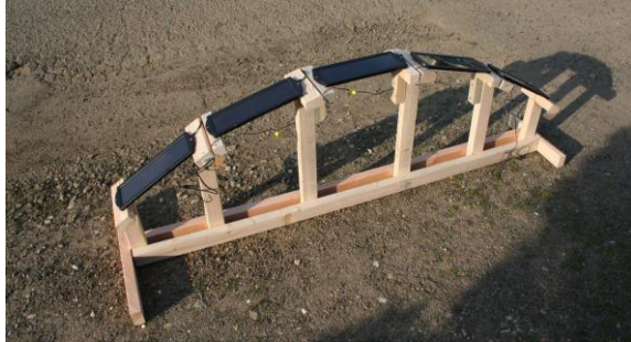
Figure 3. Flat (top) and curved profiles with five solar panels wired in series
