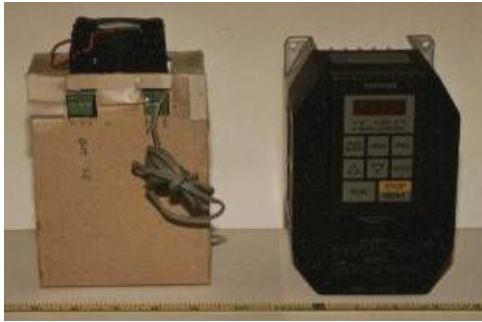
Figure 15. Comparison of the developed inverter (left) with a commercial one
