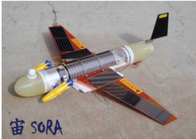
Figure 1. Solar-Powered Underwater Glider, SORA Note. From “Development of a Solar-Powered Underwater Glider,” by M. Arima, T. Okashima, and T. Yamada, 2011, Proceedings, IEEE Symposium on Scientific Use of Submarine Cables and Related Technologies , pp. 1-5. Reprinted with permission.
