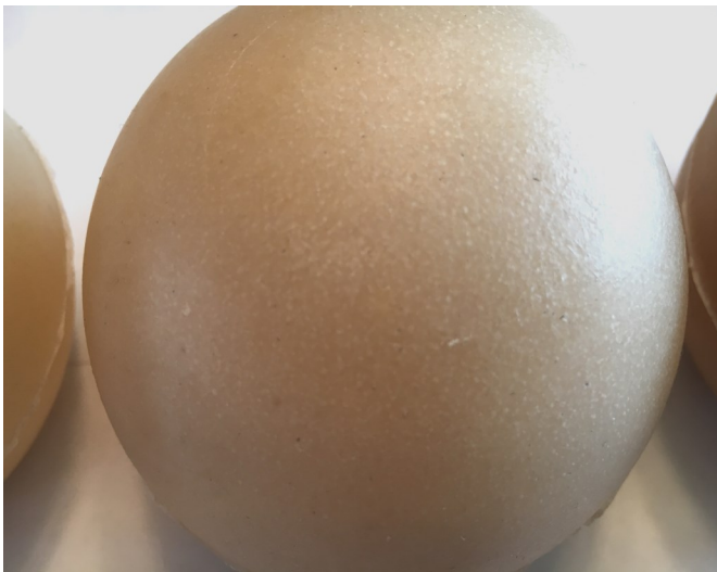
Figure 8. Samples with 7.5% Filler and Having Small Pinhole Voids over Their Entire Surface
