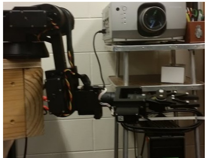
Figure 18. Robotic Arm Bends Elbow until Parallel to the Floor
