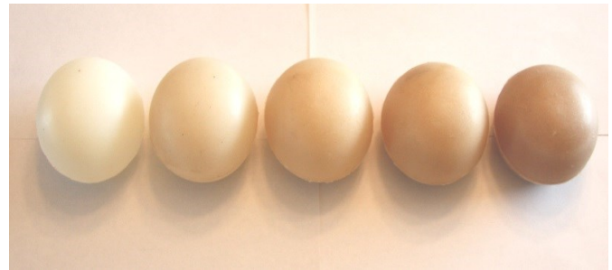
Figure 4. Samples Produced with 0%, 2.5%, 5%, 7.5%, and 10% Fiberglass/Polyester Powder (left to right)
