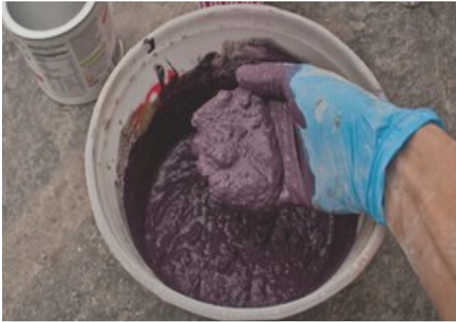
Figure 3. Incorporation of PVA Microfibers in Concrete
