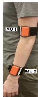
Figure 1. Subject Wearing the Two Inertial Measurement Units (IMUs)
