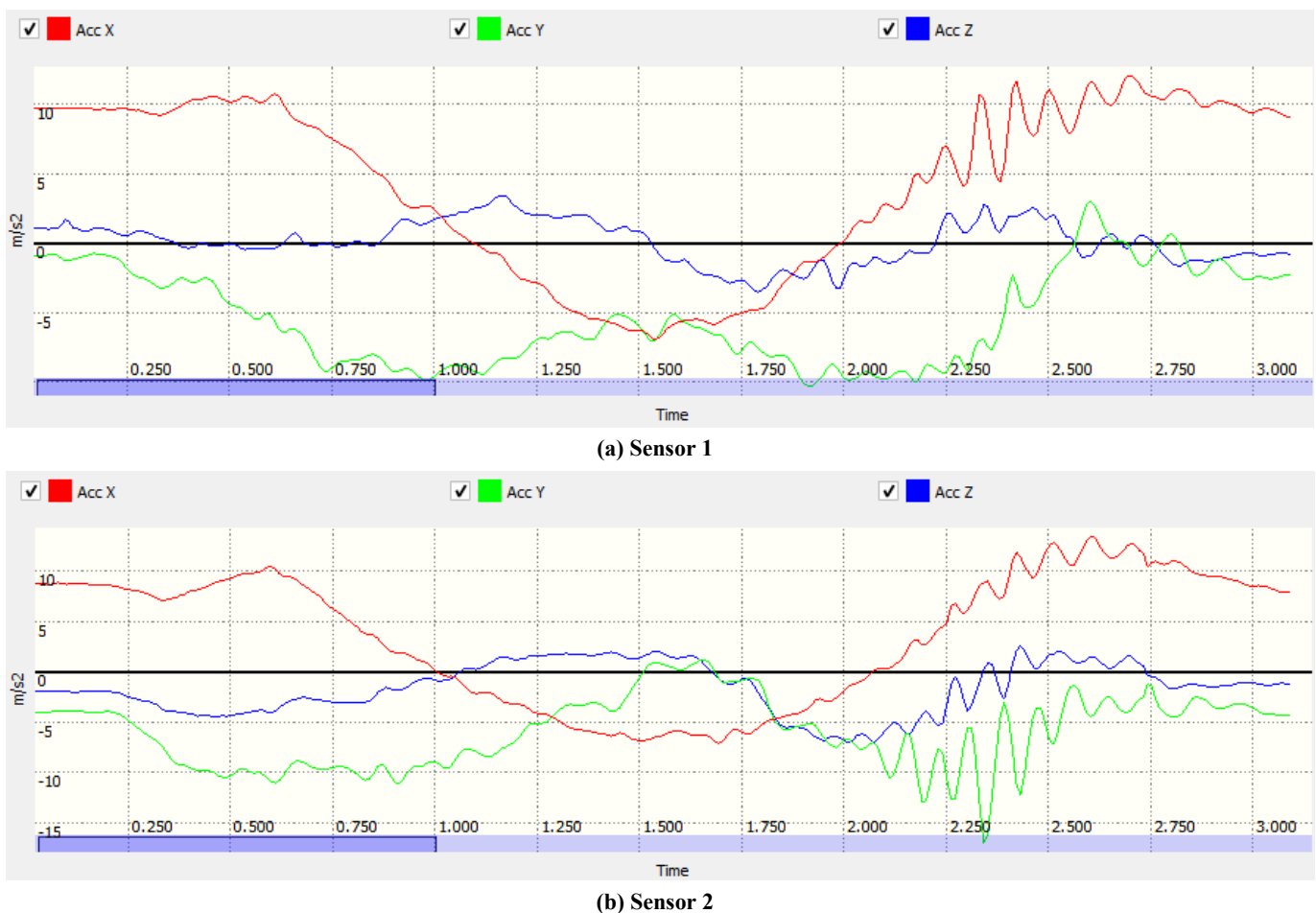
Figure 9. Acceleration Waveforms for Counterclockwise Windmill
