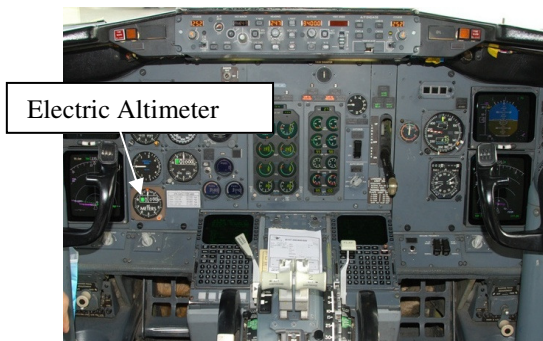
Figure 2. A view of the instrument panel at the flight deck of a B737
