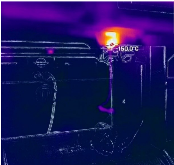
Figure 12. Material run-out condition. Note that the extruder is warm but there is no extrusion of material—old material is losing heat.
