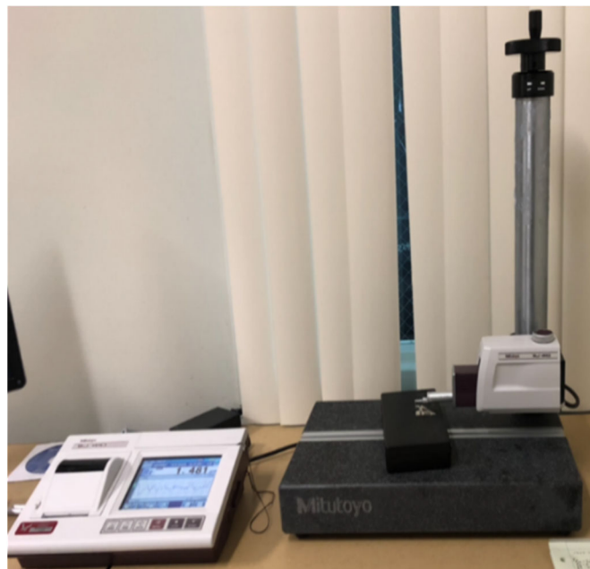
Figure 1. Profilometer setup used in the experiment. Mitutoyo surface roughness tester SJ – 410.
