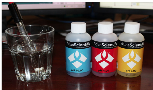
(c) pH calibration solutions and test water
