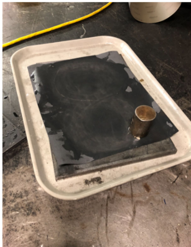
(b) Mounting the sample to a 0.875-lb rod and sanding in a figure-8 pattern.
