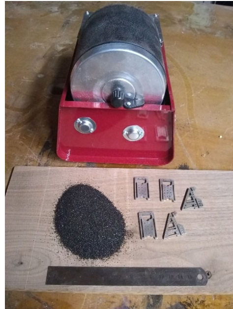
Figure 7. Tumbling setup and media used.
