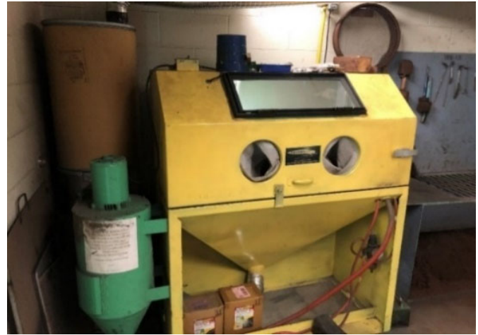
(a) Sandblasting setup used.
